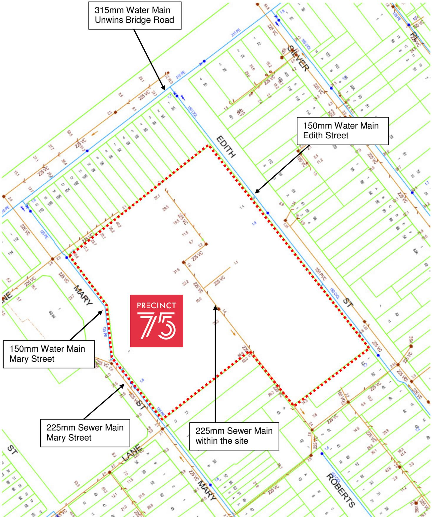
Figure 9 - Water & Sewer Plan (Source: Sydney Water)
